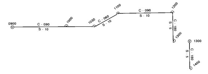
Figure 703. A typical dead reckoning plot.
